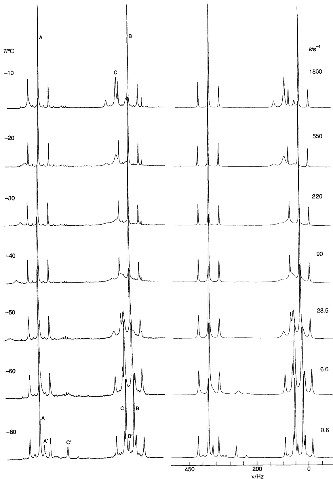
Fig. 5 250 MHz ^1\text{H} NMR spectra (Pt-Me region) of [\text{PtMe}_3(\text{terpy})] in \text{CD}_2\text{Cl}_2 at low temperatures showing the effects of arresting the rotation of the pendant pyridine ring. Computer simulated spectra are shown alongside. At -80^\circ\text{C} , the signals A, B, C refer to the major rotamer and A', B', C' to the minor rotamer
